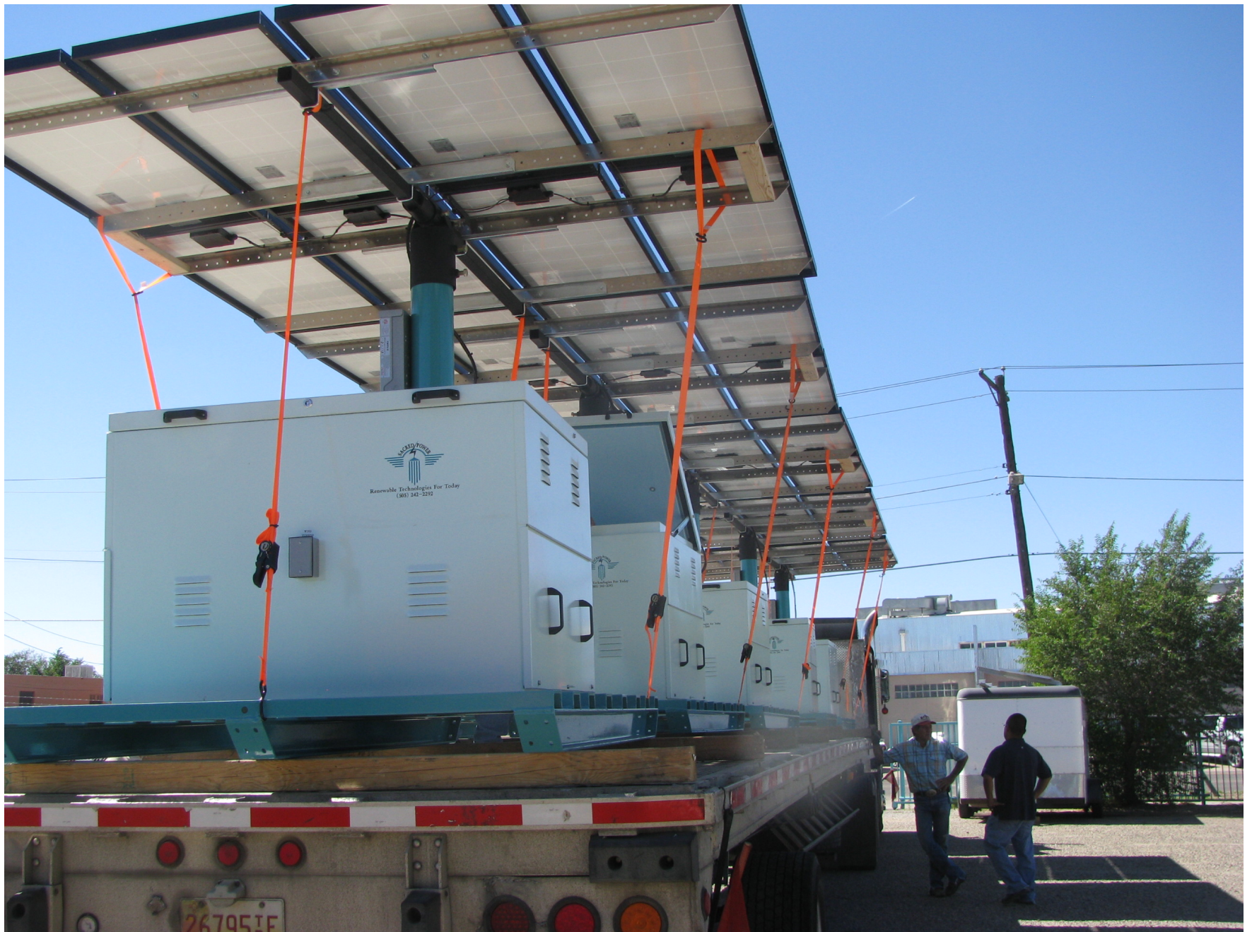
Sacred Power PV Refrigeration Systems on Flatbed
