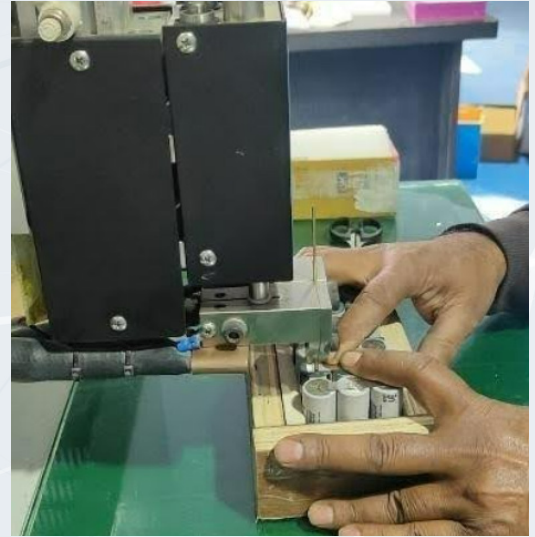
Figure 5: Spot welding of selected cells
