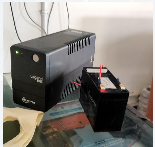
Figure 10: Test configuration of the 650 VA UPS used to assess the performance of refurbished lithium-ion batteries under backup power conditions.
