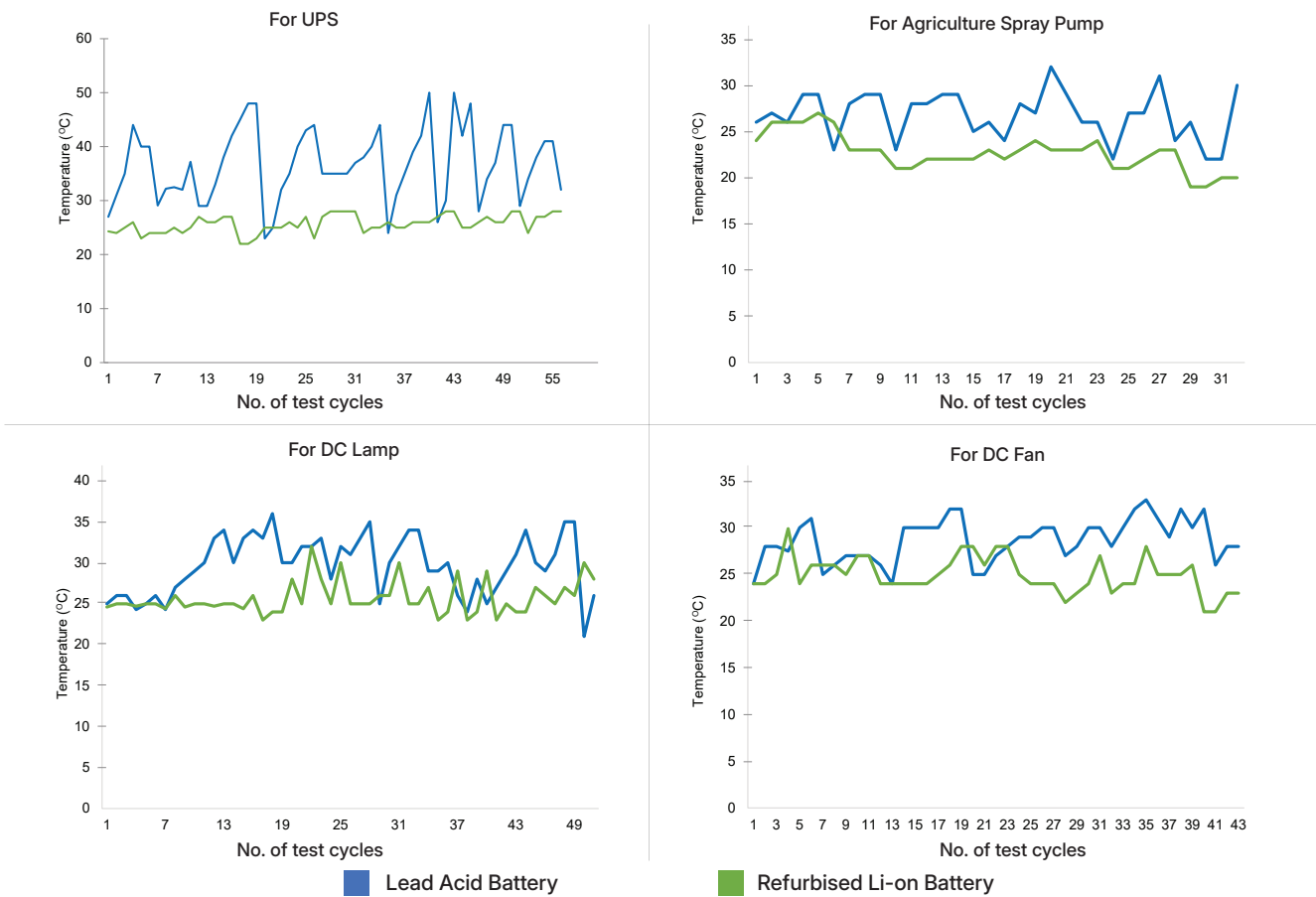
Figure 13: Analysis of the comparison of temperature between lead acid battery and refurbished lithium-ion battery.
