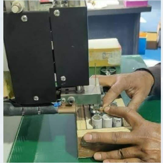
Figure 5: Spot welding of selected cells
